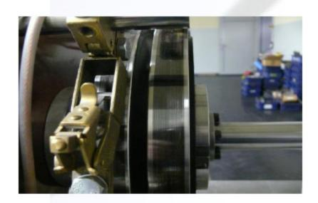
Poor brush contact results in voltage spikes and potential ring and bearing damage
